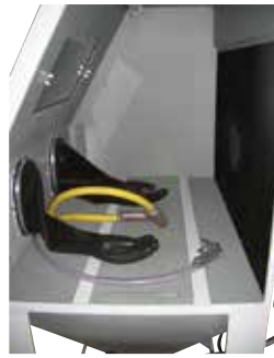
Blasting and compressed air gun
